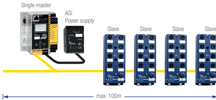
Config. A1: The standard: Single network, often with coupling to a higher-level network, e.g. to PROFIBUS
