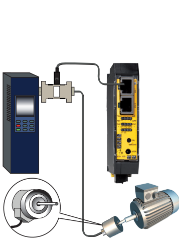
Encoder signal between encoder and converter is tapped.
